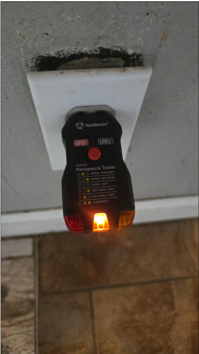
6.3 Item 4(Picture) Ungrounded outlets throughout the house. A qualified electrical contractor should find and fix any and all National Electrical Code deficiencies.
